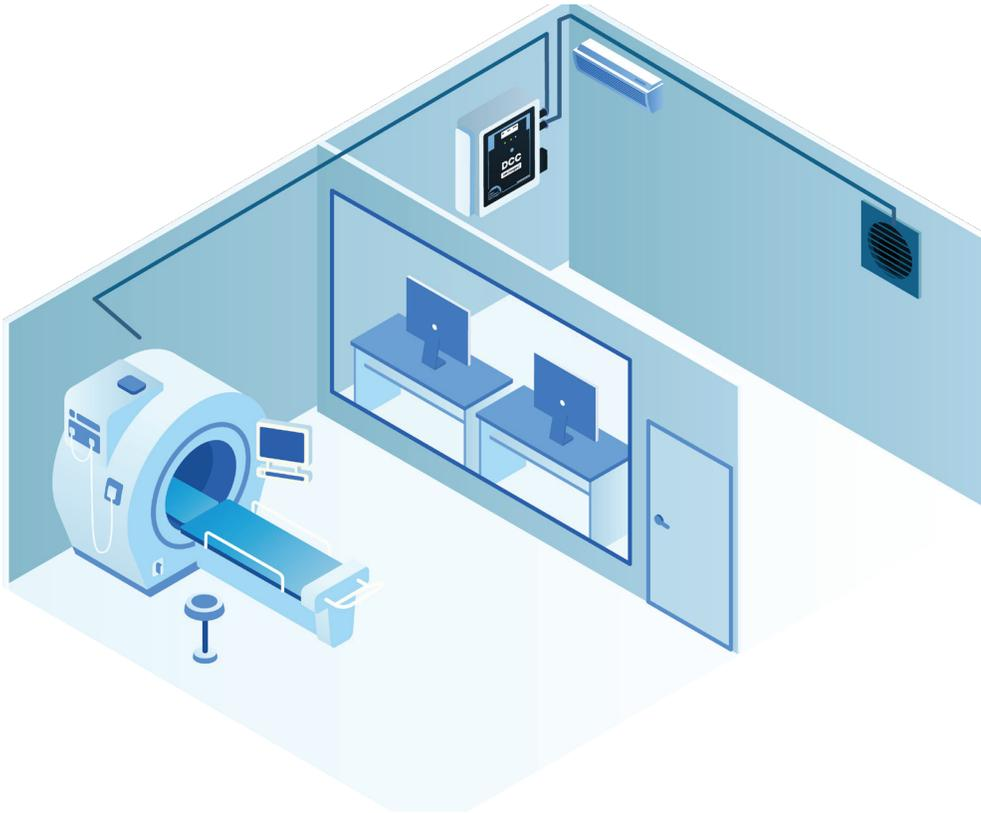
likely to occur. The air in the area is continuously drawn into the DCC-MRI device by a sample draw pump, flowing over the sensor and is exhausted through the outlet port. If the Oxygen level drops below a specified set point, the DCC-MRI will go into alarm.
