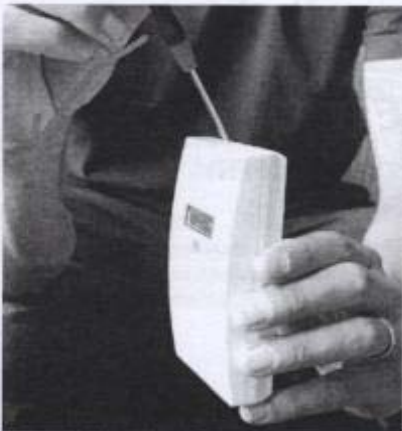
Figure 2. Closed housing seen from the side. The housing is opened by inserting a screw driver and pushing left (to the front side) The locking hooks will then be released.
