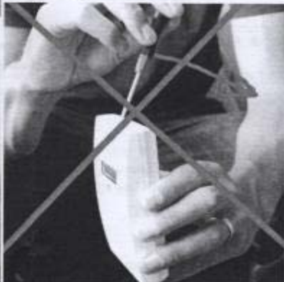
Figure 3. Closed housing seen from the side. Never push to the right. The locking hooks may break and the housing is damaged
