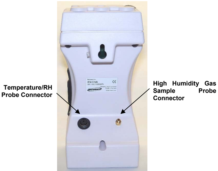
Figure 10-1. YESAIR for Dual-Probe Applications
