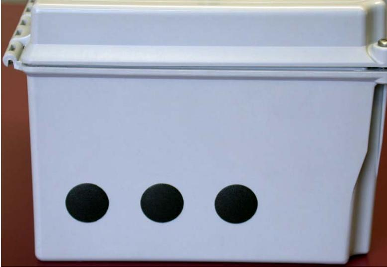
Three conduit entry openings, for 1/2" conduit, have been provided along the bottom edge of the system enclosure. See photos above (with protective plugs inserted) and below (with plugs removed). To access the openings, remove the protective plugs. If a fourth opening is required, it will have to be drilled on site. Take caution to avoid damaging internal components when drilling any holes in the enclosure.
