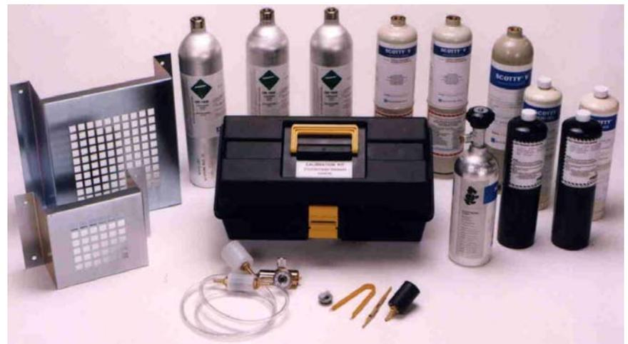
Calibration kits, gases and metal protective guards
